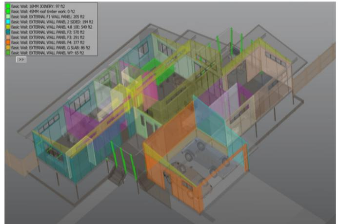
There can also be differences in the measurement of the floor area of a building, which can throw off comparisons by at least a few percentage points. In different regions, the enclosed area of a building might be measured to the exterior face of external walls, to the mid-point of the wall, or to the inner face. There can also be differences between how covered-not-enclosed areas are treated, and in what size of floor openings should or should not be deducted.
